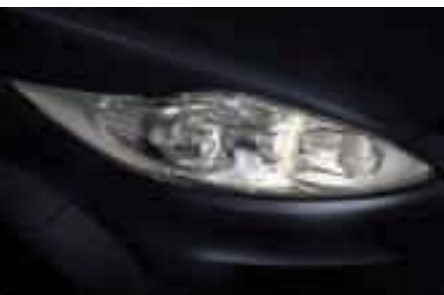
Halogen projector headlights Produce a stronger beam. (Standard)
