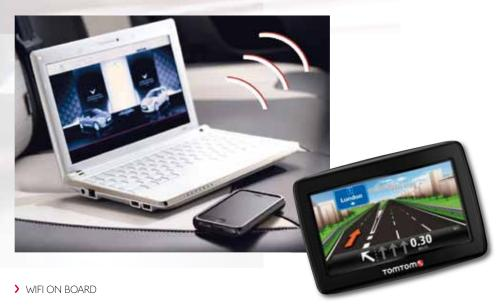
Citroën's 'WiFi on Board' system creates an in-car wireless network, allowing simultaneous internet connection for multiple WiFi devices such as laptops, smartphones and game consoles.
