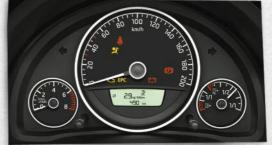
On all Citigo models the central feature is a **large speedometer**. The SE, Sport and Elegance dials (shown here) also feature a **rev counter** and a fuel gauge. S models features a digital fuel gauge.
