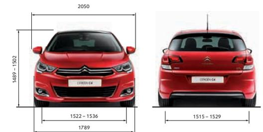
All measurements are in millimetres.
