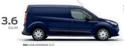
Max. gross payload\* up to 834 kg Gross vehicle mass from 2,165 kg to 2,405 kg
