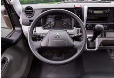
An infinitely adjustable steering wheel and dash-mounted shifter give drivers more control, while instruments and displays are always within easy reach or view. By moving the shifter off the floor, we create more leg room and easier access for passengers with full traversability from left or right for safer entry & exit.
