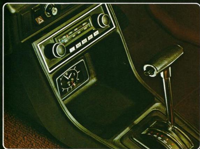
Automatic transmission – only available with a 1600cc engine on the Escort Ghia – and the push button radio are factory fitted options available at extra cost.
