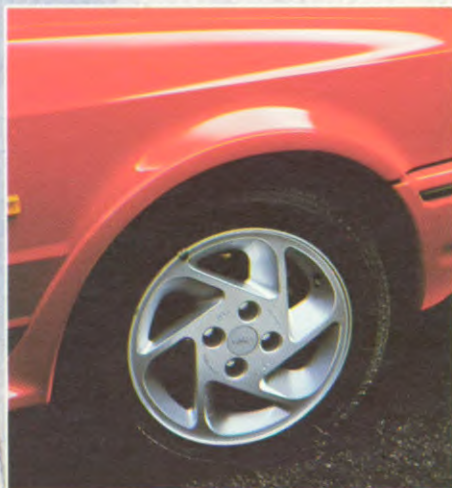
The light alloy 6 x 15 wheels fitted with 195/50 VR 15 tyres, providing large reserves of grip for sure-footed cornering and razor-sharp handling are standard on the Escort RS Turbo.
