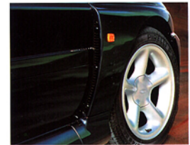
Above: Air extraction grilles in the front fenders contribute to engine cooling.
