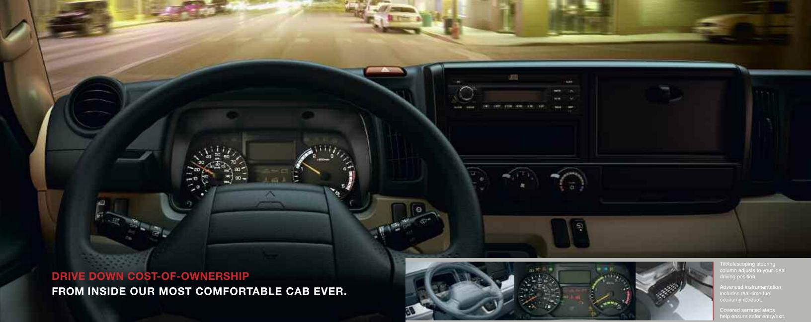
Once you sit behind the tilt/telescoping wheel of a Canter work truck, it hits you. The new interactive instrument cluster features DEF level monitor, a multi-information display with selectable readouts including real-time fuel economy, DPF gauge, and much more.
