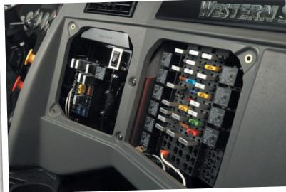
**STAY IN THE WOODS.** You work your trucks hard, so sometimes they need a little attention. Stars are designed for incredible durability and serviceability, with features like Grade 8 frame fasteners and in-dash power distribution modules so you can make quick repairs in the field and keep on working.
