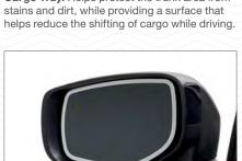
**Auto-Dimming Exterior Mirrors with Approach** Light. Designed to enhance nighttime driving safety by reducing headlight glare. When you approach the vehicle or unlock the doors with the keyless entry system, LED lights in each exterior mirror illuminate the ground next to, and towards the rear of, the vehicle. During nighttime driving, the Auto-Dimming Exterior Mirrors dim in unison with the Auto-Dimming (Interior) Mirror when glare is detected.
