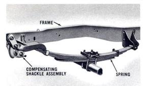
\*ALL-NEW FLEX-O-MATIC REAR SUSPENSION — Unique load compensating shackles automatically shorten the leaf springs in direct proportion to the weight of the load. Teamed with Ford's exclusive Twin-I-Beam front suspension, the all-new Flex-O-Matic rear suspension provides the smoothest, most stable ride in the history of light trucks loaded or unloaded. Optional on the F-100.
