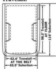
The difference in length of Suburban's and Travelall's cargo deck behind the driver's seat is nearly a foot and a half—all in Suburban's favor.
