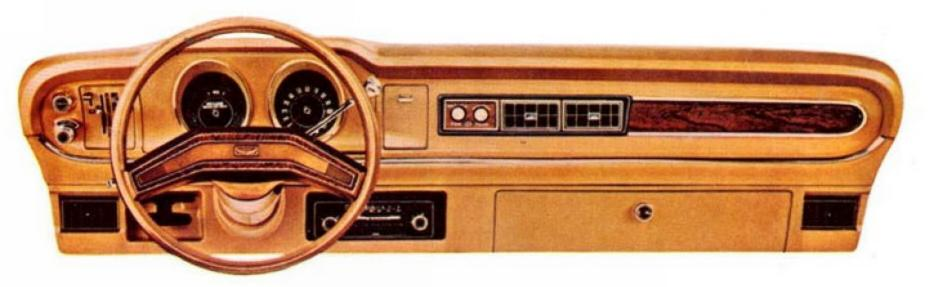
Installs in most models. Same cooling capacity as custom models. Controls located for easy driver reach. Choice of three blower speeds and full temperature selection.
