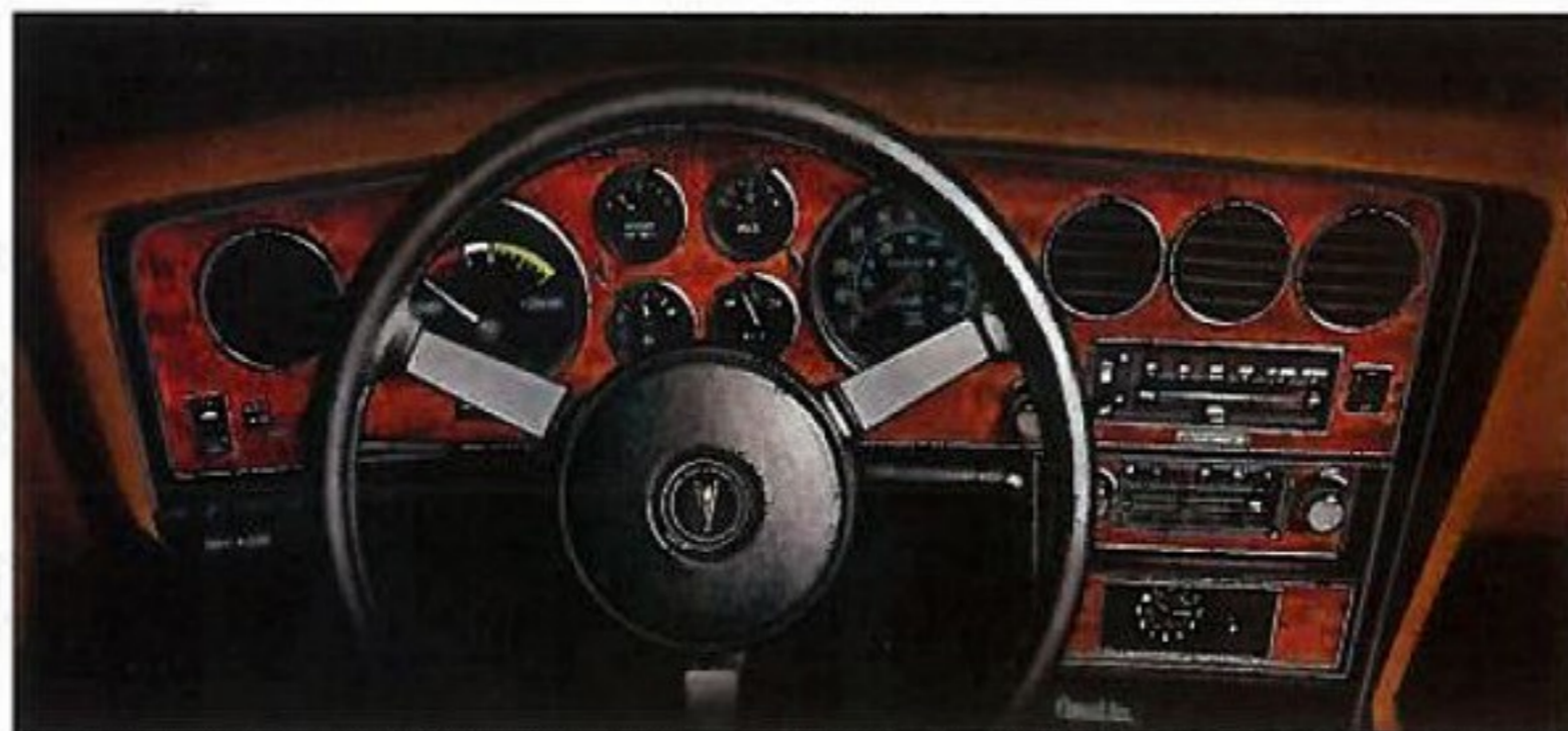
Grand Am instrument panel with standard rally gauges, custom sport wheel and available economy gauge.
