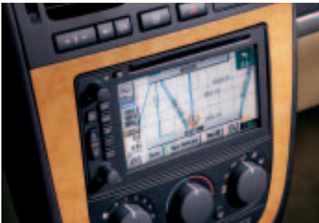
GPS navigation 1 radio. Uses GPS and a mapping DVD to visually and audibly tell you how to get from here to there. A CD player and radio are also integrated into the system. (Interim availability)
