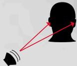
Unlike with high-frequency sounds, the brain cannot detect where low bass frequencies are coming from, making it seem as if the sound is hitting both ears at the same time. Because of this, Bang & Olufsen® sound engineers only had to design one custom-fitted subwoofer to reproduce the kind of deep, cabin-filling bass that brings music to life.
