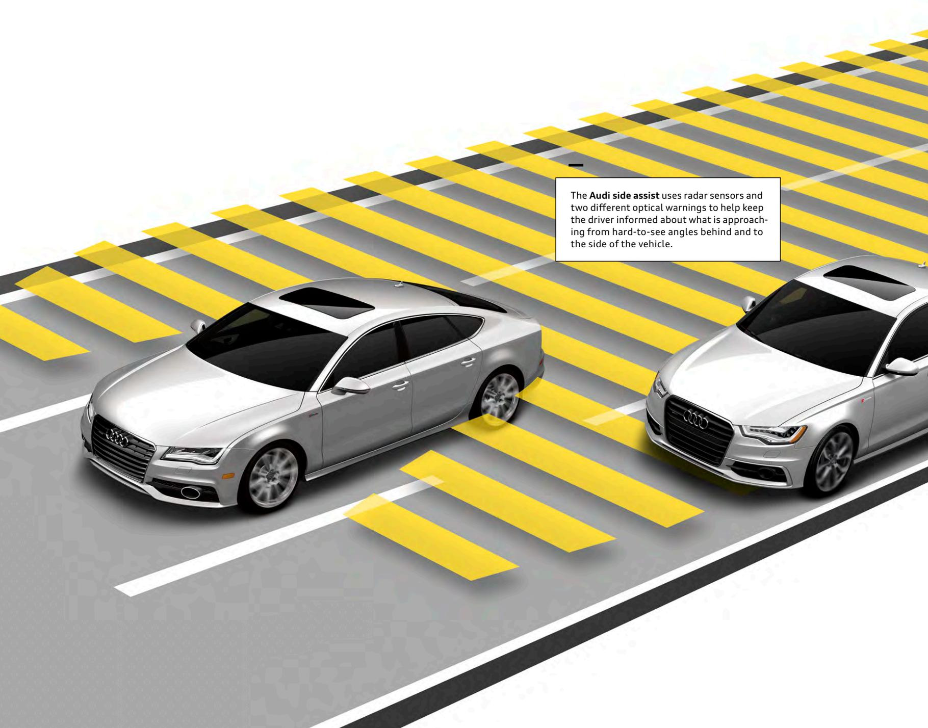
The **Audi side assist** uses radar sensors and two different optical warnings to help keep the driver informed about what is approaching from hard-to-see angles behind and to the side of the vehicle.
