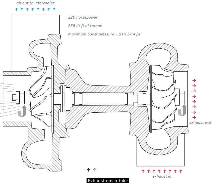
Exhaust from the engine spins the turbine that is connected by a shaft to a compressor that pressurizes air. The compressor forces this pressurized air into the cylinders at boosted pressures up to 17.4 psi, thus producing more power from a smaller displacement engine.
