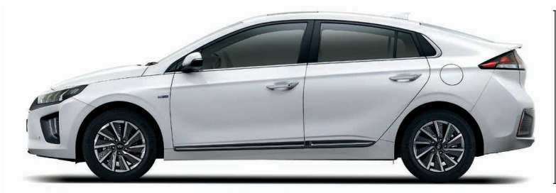
Wheel base 2.700 mm Overall length 4.470 mm Overall height 1.475 mm
