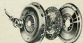
Heavy-Duty Clutch (10¾-inch). For use in place of the regular 9¾-inch clutch of 3100 Series models and the Sedan Delivery. Increases facing material area by 45 per cent, prolongs its life. Recommended for vehicles in multi-stop delivery service.
