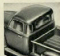
De Luxe Cab. Rear corner windows, bright metal windshield and window reveals, garnish moldings, driver's arm rest, right-hand sun shade and seat back trim panel. Chrome grille, 3000 series.
