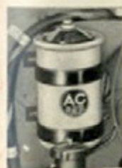
Oil-Filter. Protects engine bearing surfaces, by removing dirt and grit from the engine oil.
