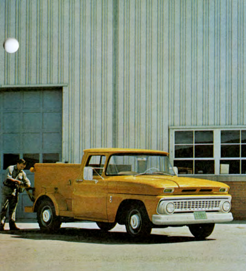
CHASSIS-CAB MODEL C1403 (with special utility body)—Seven light-duty chassis-cab models offer broad coverage of the ½- to 1-ton field, with optional equipment and ratings available for every job requirement. And new frames make every type of body easier to install.
