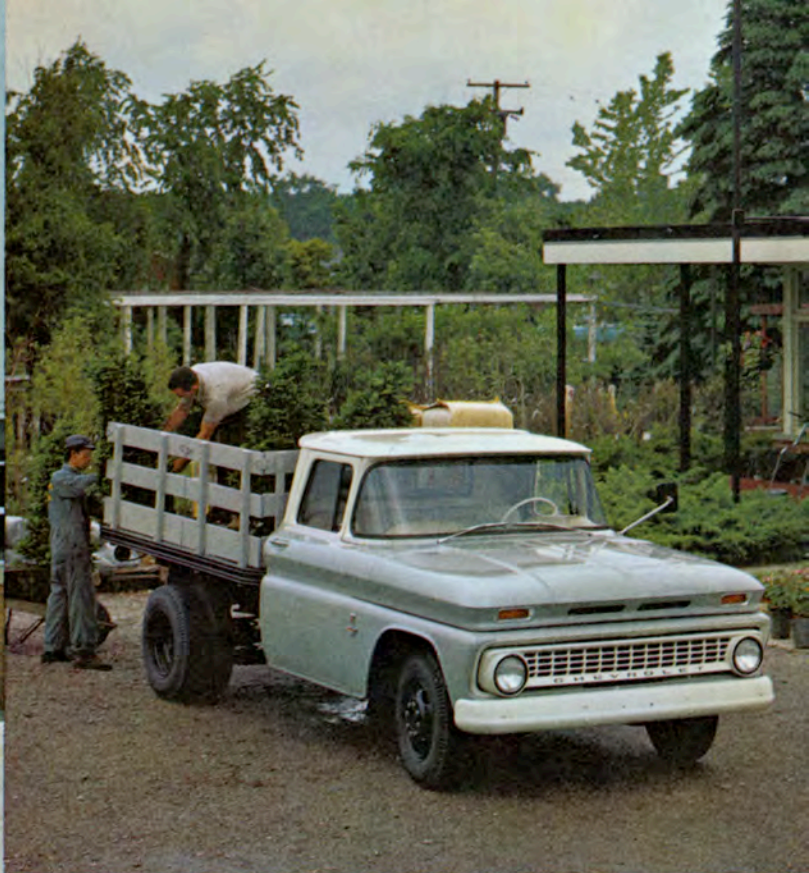
STAKE MODEL C2509 (with new dual rear wheel option)—Three light-duty Chevy stake models offer a better answer for bulky cargoes for every job in the 5,500- to 10,000-lb. GVW range. C2509 and 3609 carry 8- and 9-foot bodies, respectively, featuring top-quality construction throughout.
