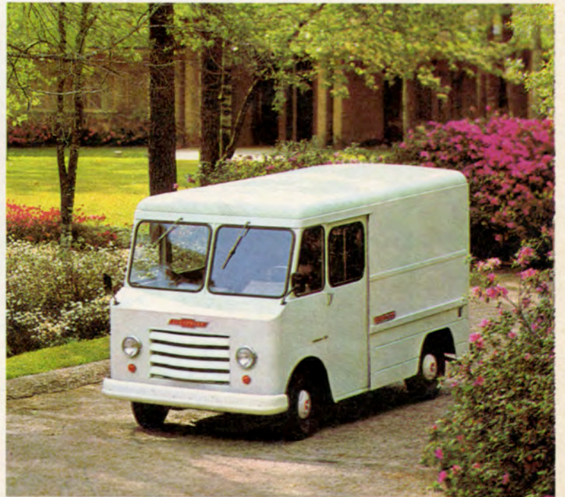
STEP-VAN 7 — This is Chevrolet's smallest Step-Van, available in four different body sizes and powered by a gas-saving 194-cubic-inch Six.*
