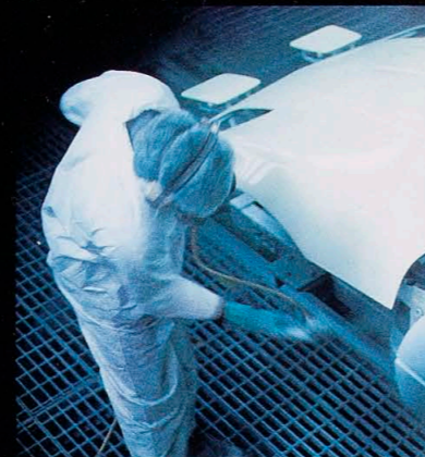
One-piece hood/fender assembly eliminates seams.
