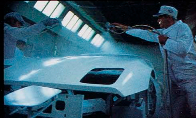
New Corvette gets its first color coat.
