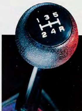
Five-speed manual transmission with overdrive available on all S-10 Pickups.
