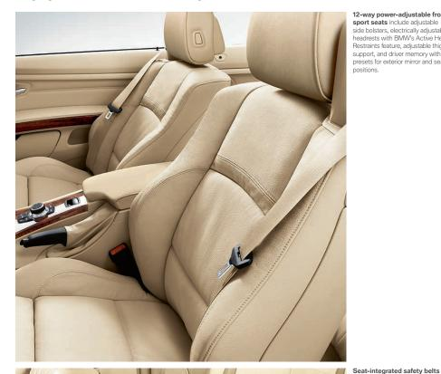
12-way power-adjustable front sport seats include adjustable side bolsters, electrically adjustable headrests with BMW's Active Head Restraints feature, adjustable thigh support, and driver memory with two presets for exterior mirror and seat positions.
