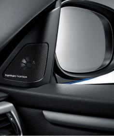
Harman Kardon<sup>®</sup> Surround Sound Audio System with vehicle-specific equalizing and powerful 340W amplifier. The 11-speaker system includes four tweeters, two midrange speakers located in the door panels and two midrange speakers located under the rear shelf space, two bass speakers located under the front seats and one midrange center channel speaker located in the dashboard.
