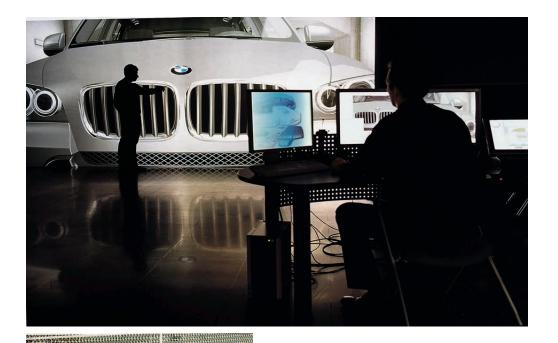
In addition, VR enables the early assessment of design alternatives. Each design can be visually represented, evaluated and compared. A 3-D model is generated based on the design. To do this, the computer subdivides the vehicle into tiny triangles, or polygons, placing over the design a virtual grid that describes the vehicle's geometry.
