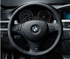
Three-spoke, leather-wrapped multi-function M sport steering wheel , included in the M Sport Package and 335is, provides excellent grip, with its thicker, leather-wrapped rim and pronounced thumb profile.
