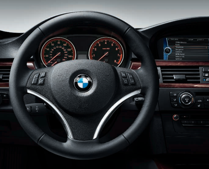
Three-spoke leather-wrapped multi-function sport steering wheel lets you keep both hands on the wheel while adjusting various comfort functions, such as changing the radio, CD selections and volume.
