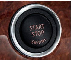
Engine Start/Stop button 1 and key fob control the engine. Upon inserting the key fob into the starter switch slot, and the electronic identification system confirming that it is the correct key fob, the engine can be started (or later, shut off) by pressing the Start/Stop button.
