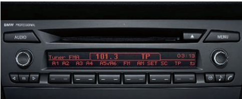
BMW anti-theft AM/FM stereo CD/MP3 player audio system includes Radio Data System (RDS), Auto-Store, and 3-channel FM diversity antenna, as well as reads and displays song title and other information. HD Radio TM receives free, digital AM/FM broadcasts across the U.S. in clear, static-free quality sound – AM sounds like FM; FM sounds like CD. Also enjoy "multicast" FM stations, as well as a variety of innovative data services. For more information on HD Radio receivers and to find HD Radio AM/FM stations near you, visit HDRadio.com .
