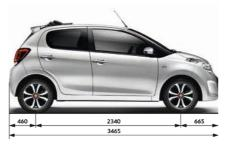
All measurements are in millimetres.
