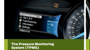
Pressure is measured in all the road tires. When any tire is significantly underinflated, a telltale on the instrument panel alerts you. That's the signal to check the pressure of each tire, matching the figure to the psi (pounds per square inch) recommended for the vehicle.
