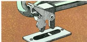
Quick release seats. Now Sportvan converts from people- to cargo-carrying in minutes. Both standard and available bench seats are secured to the floor by cam-type front latches and hooked rear retainers that fit onto anchor pins. When the latches are released, as shown above, the seat can be slid off the rear anchors. then lifted and removed. Simply reverse procedure to reinstall.
