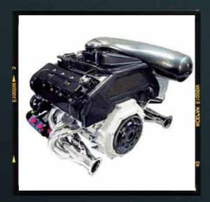
The air intake system incorporates a large centrifugal supercharger. It is connected to a custom-built intercooler which lowers the charged intake air temperature from 150°C to 50°C. A specially manufactured dry-sump engine lubrication system enables a
