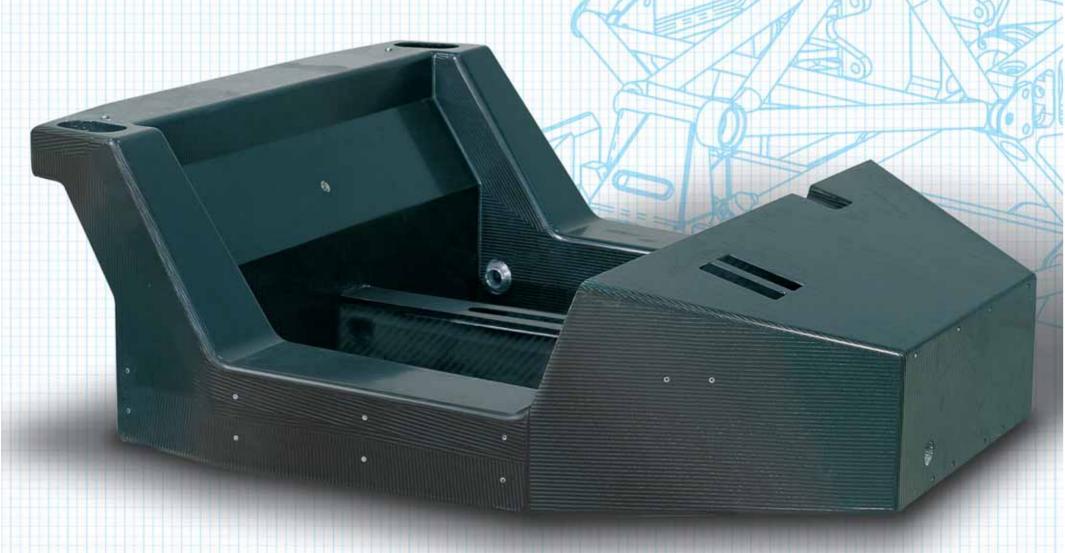
The monocoque is handmade and consists of 21 layers of carbon fibre with honeycomb in between. Thanks to the use of carbon fibre, the weight of the chassis module is only 62 kg (136 lb.) and the torsional stiffness is 28.100 Nm/degree. The monocoque gives the driver and passenger excellent protection and provides greater rigidity than any competitor, which is important for the car's handling qualities.
