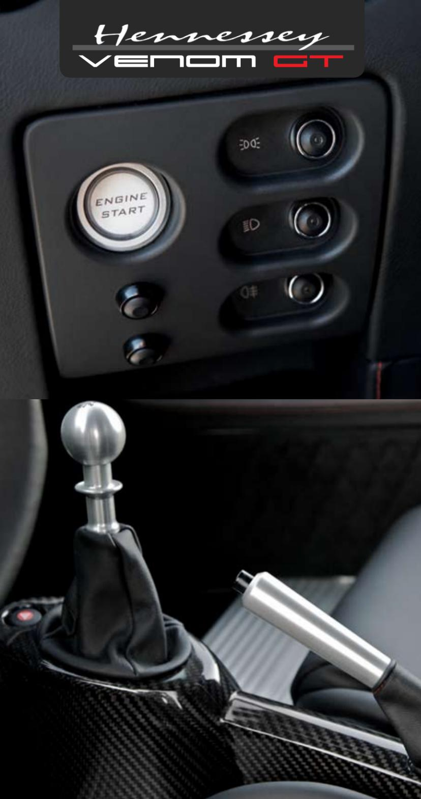
All components aboard the Venom GT are built for purpose, not flash. Lightweight carbon fiber surrounds an alloy shifter that actuates a Ricardo 6-speed manual gearbox. An AP Racing multi-disc clutch transfers the engine's copious power while remaining easy to modulate.
