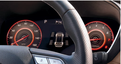
12.3" digital LCD instrument cluster
