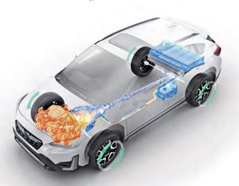
In everyday driving, the system will run on a combination of electric and gas power. It can also recover energy via regenerative braking.
