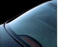
▲ SOLAR TINT GLASS. Included to filter out a higher percentage of the sun's rays than standard tint or clear glass to reduce air-conditioning cooldown times. Also helps to protect fabric surfaces from sun fading.
