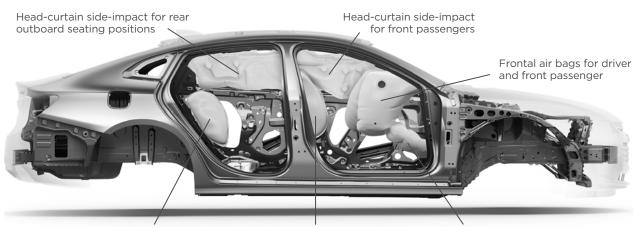
Side-impact seat-mounted for rear outboard seating positions
