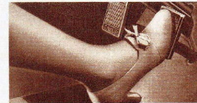
LaSalle's hydraulic brakes respond to light toe pressure. Moulded linings are moisture-proof.
