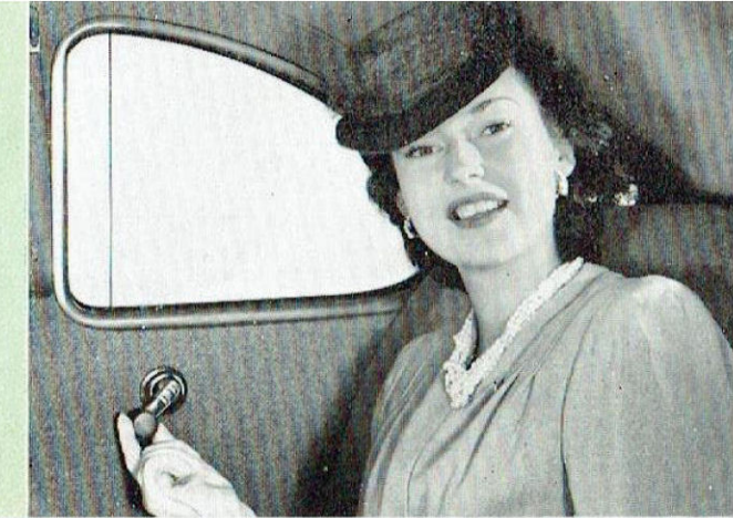
Rear quarter ventilation of the draft-free, sliding type is operated by a convenient crank.
