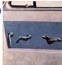
Door and window controls are nestled in the recessed panels. Inside push-button locks, when in use, give added security by making inside and outside door handles inoperative. Outside door handles are streamlined push-button type, with no open ends.
