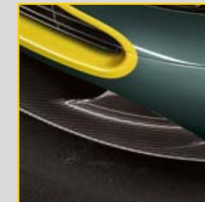
Carbon-Fibre front splitter
