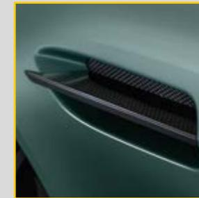
Carbon-Fibre side strakes
