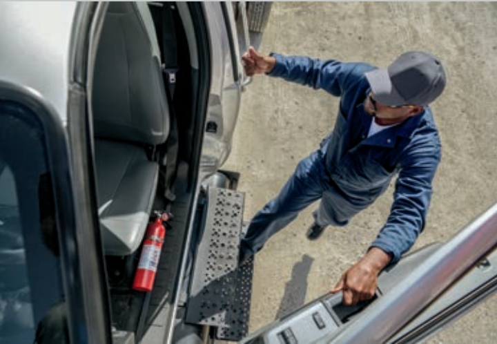
CAB STEPS AND GRAB HANDLES HELP DRIVERS ENTER AND EXIT SECURELY Standard
