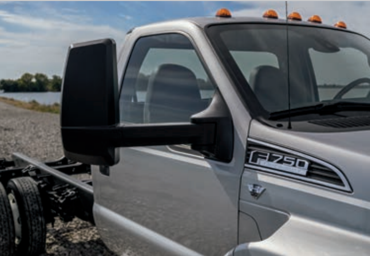
DUAL MANUAL-FOLDING, HEATED, SAIL-TYPE MIRRORS INCLUDE INTEGRATED SPOTTER MIRRORS AND CAN REACH UP TO 102" WIDE Available
