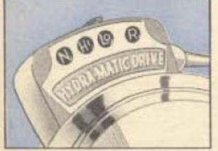
ONE of the big factors of safety in mountainous country is the ability to use the compression of the engine as a brake in descending hills. Oldsmobile's Hydra-Matic Drive provides a special "Lo" speed for this purpose. At any car speed below 40 M.P.H., you can flick into "Lo" from "Hi" without taking your hands from the wheel—
