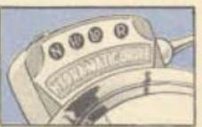
in "Hi," it is not necessary to move the lever for starting, stopping, or accelerating. The third position is marked "Lo." This speed is
