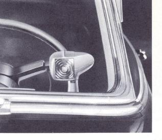
Mounted on the instrument panel at the left side of the windshield, Oldsmobile's new Autronic Eye picks up the headlight beams of approaching vehicles and automatically switches your lights from bright to passing beam. Streamlined and compact in design, it is in keeping with the smart styling of the new 1952 interiors.
