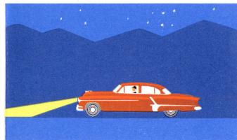
As soon as an oncoming vehicle comes within range, the Autronic Eye picks up the headlight beam and actuates the relay switch which instantly dims your headlights.
