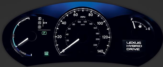
In ECO mode, the throttle response is modified and climate control is optimized for efficiency. In EV<sup>1</sup> mode, the CT can run on battery power alone for short distances, at low speeds under certain conditions. Because the gasoline engine is not engaged, noise is minimized and emissions are eliminated. Depending on driving conditions, both settings can noticeably reduce fuel consumption.
