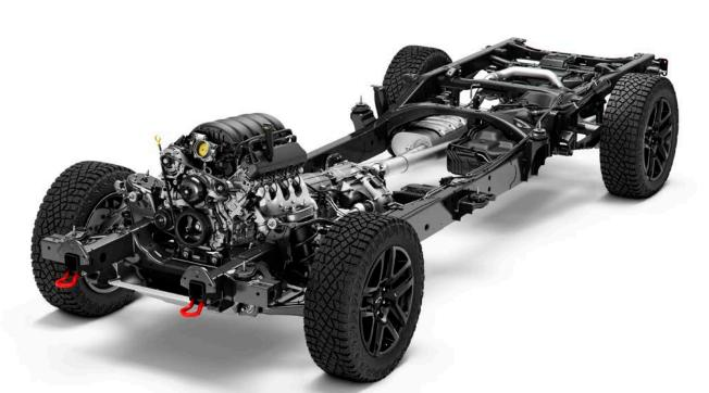
The independent short/long arm front suspension provides excellent wheel alignment, ride comfort and tunability with reduced weight. The live axle rear suspension includes 2-stage, semi-elliptic multileaf springs to strike a balance between payload management and ride quality.
