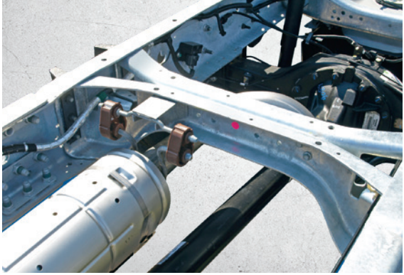
Available Galvanized Frame System (Optional for the 19,500 lbs. GVWR and 22,000 lbs. GVWR with 208" WB)
