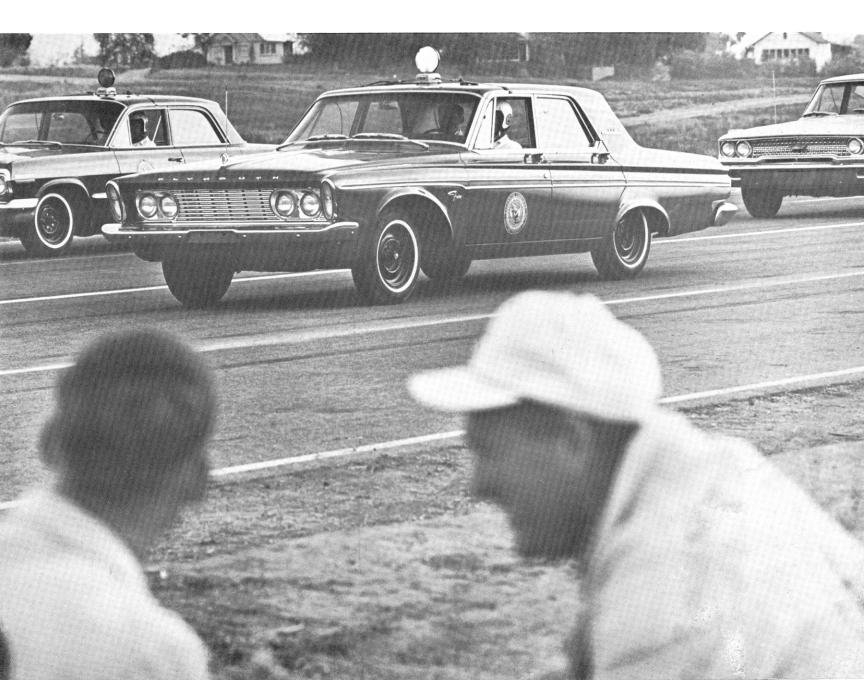
**QUARTER-MILE RUN** Here the tempo picks up. Another test of acceleration from a standing start, but this time over a longer stretch. A car needs more than quick response here; it needs stamina as well. Electronic equipment is ready on the backstretch. As each car crosses the finish line, the electric eye blinks and elapsed time is recorded automatically. Again, each car is run individually. Again, the three drivers get a crack at each car. Again, Plymouth comes home first,
