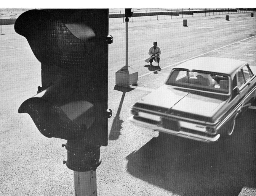
**EMERGENCY STOP** This is a test of braking ability. Each car races down the backstretch until it reaches a speed of 60 miles per hour. At that instant, the driver hits the brakes. NCTI officials arrive at the results by measuring the skid marks from one end to the other. After three runs for each car, with a different driver at the wheel for each run, the official average figures give Ford its
