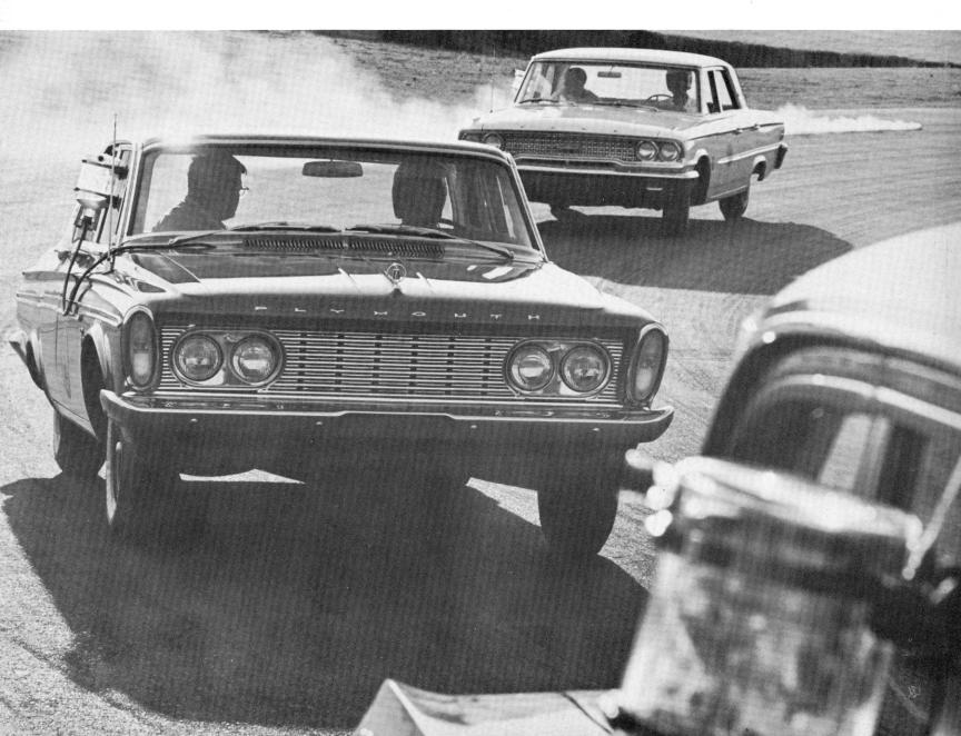
HILL CLIMB For this next event, the test cars move off the asphalt of the track to the base of a steeply inclined, dirt-covered hill. (NCTI officials calculated the grade at 12%.) With the cars at the bottom of the hill and the timing equipment at the top, the object is to roar to the top of the slope in the quickest possible time. Once again, the cars are run individually and drivers rotated. When the
