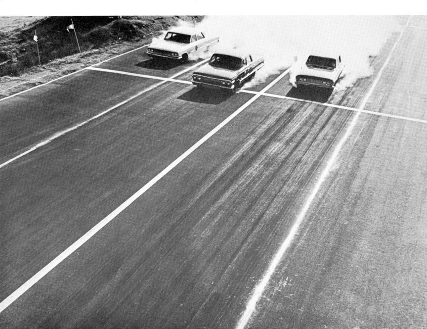
**ECONOMY RUN** Now it's time to put a price on all this performance. First, the gas is drained from each test car. Then, exactly two liters of regular gasoline (slightly more than half a gallon) are poured into a bottle for each car, and fed to the fuel pump through a hose. The drivers are instructed to maintain an average speed of 45 miles per hour, which means well over 60 mph on the straightaways to compensate for reduced speeds on the turns. As each car's engine dies, the driver
