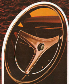
Deluxe steering wheels make it. Three spokes with partial horn ring. Spokes padded with foam, and covered with special-grained butyrate. For a luxury look that really makes it.
