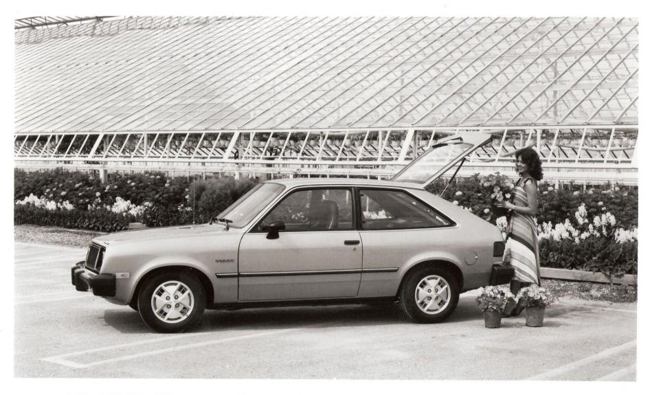
1982 PONTIAC T1000 ... A five-speed manual transmission is available on 1982 Pontiac T1000 three-door hatchback models and new cast aluminum wheels (shown) are optional on all T1000 models. Preliminary EPA fuel economy ratings on the standard 1.6-liter four-cylinder engine with a five-speed transmission are 30 and 43 miles per gallon in city and highway driving respectively.
