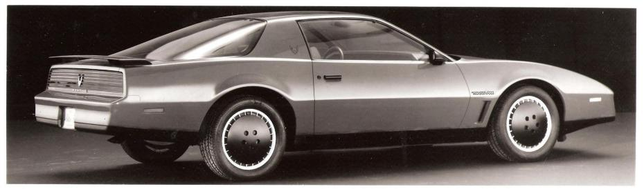
1982 FIREBIRD TRANS AM ... Powered by a 5.0-liter V-8 four-barrel engine, the 1982 Trans Am is available with four-speed manual or three-speed automatic transmission as standard equipment. Also standard on all Trans Ams is a functional wing-type rear spoiler. All 1982 Firebird models carry four passengers and have a large, contoured frameless all-glass hatch, offering improvement in cargo space and versatility.
