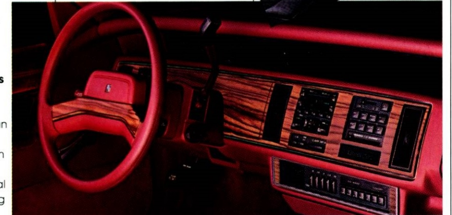
The Regal's standard instrument cluster includes a digital speedometer, rotary odometer, an analog fuel gage and aircraft-type warning lights.
